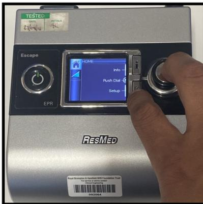
Access the clinical menu by simultaneously holding down the button with the 2 ticks ✓ and the dial for 4-5 seconds
